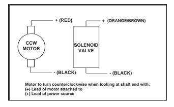
Power supply wiring must conform to all required safety codes and be installed by a qualified person. Check that supply voltage agrees with that listed on product nameplate. Minimum supply wire gage: 14 AWG.
